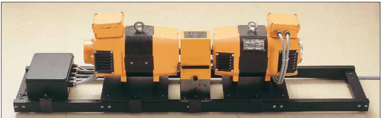
Turbine Generator Set: Power is generated by a 3-ph synchronous generator driven by a separately excited DC-motor as turbine. The electrical machines set is fully connected electrically and mounted mechanically on a machine bed.
