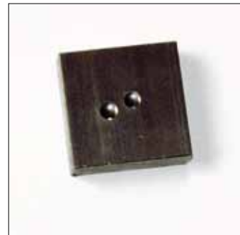
Brinell Test Piece after Brinell Indent
