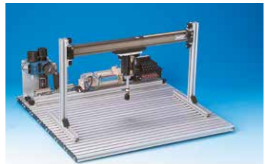
An assembled portal robot, 2 axis.
